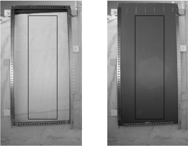
Fig. 5. Sample grayscale image of a section of a snowpit wall. The left image shows an empty frame around a snow face and the right image shows the reflectance board inserted into the frame to cover the snow face. The board is used as a reference to measure the distribution of illumination throughout the region within the frame.
