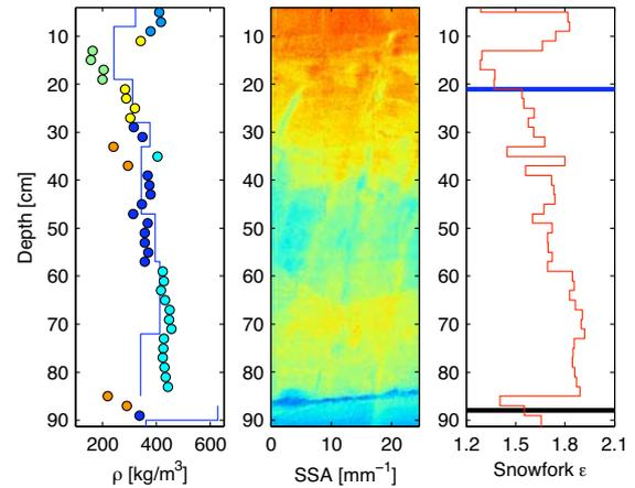
**Fig. 7.** The center panel show specific surface area varying down the profile. Independent measurements of density  $\rho$  (left panel, blue line) and permittivity  $\epsilon$  (right panel, red line) were also made. The circles on the left panel are the permittivity values converted to density. Horizontal lines on the right panel indicate ice layers: blue for a strong melt and black for what is suspected as the last summer melt layer.
