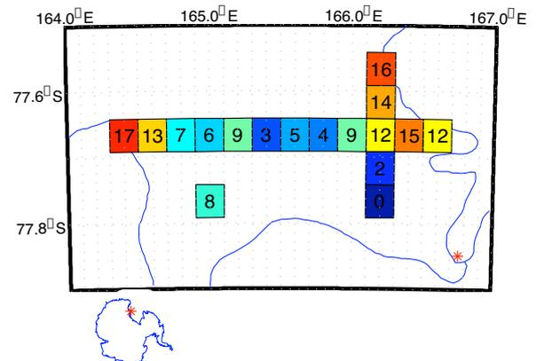
**Fig. 3.** Average snow thickness in centimeters for quadrants on sea ice where ground-penetrating radar profiles have been made. The red asterisk is the location of Scott Base. The northern east-west transect is mostly over first-year ice, except for the areas close to land. In the south, it becomes predominantly multi-year ice.
