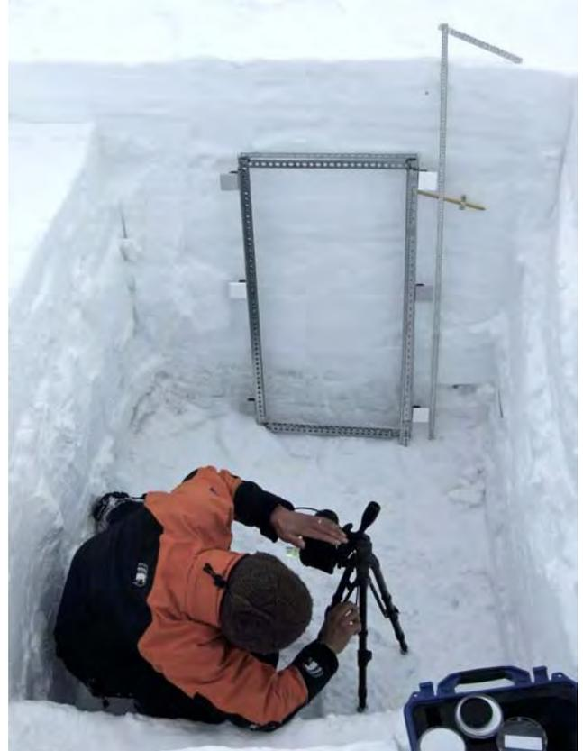
**Fig. 4.** A tripod is used to situate the camera so that it is centered around the frame and a bubble used to align it parallel to the pit wall. A ruler along the frame provides a reference for scale as well as for camera focus. Reflectance tiles around the frame serve as references for 50% (gray) and 90% (white) reflectance. Photo by W. Rack.
