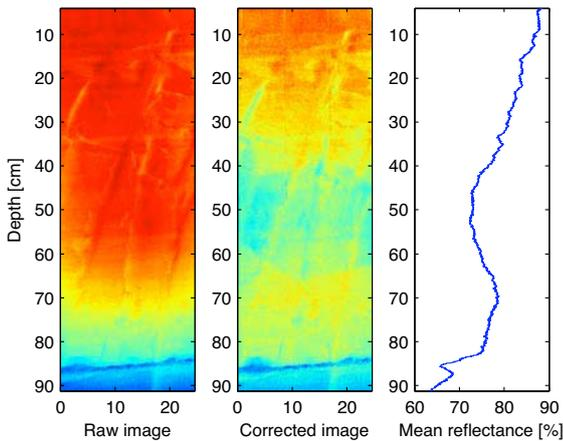
**Fig. 6.** Only the section within the black boundary on Fig. 5 is used to calculate reflectance. The left panel shows an uncorrected image while the center panel is corrected. Once corrected, the brightness values can then be converted to reflectance (right panel).
