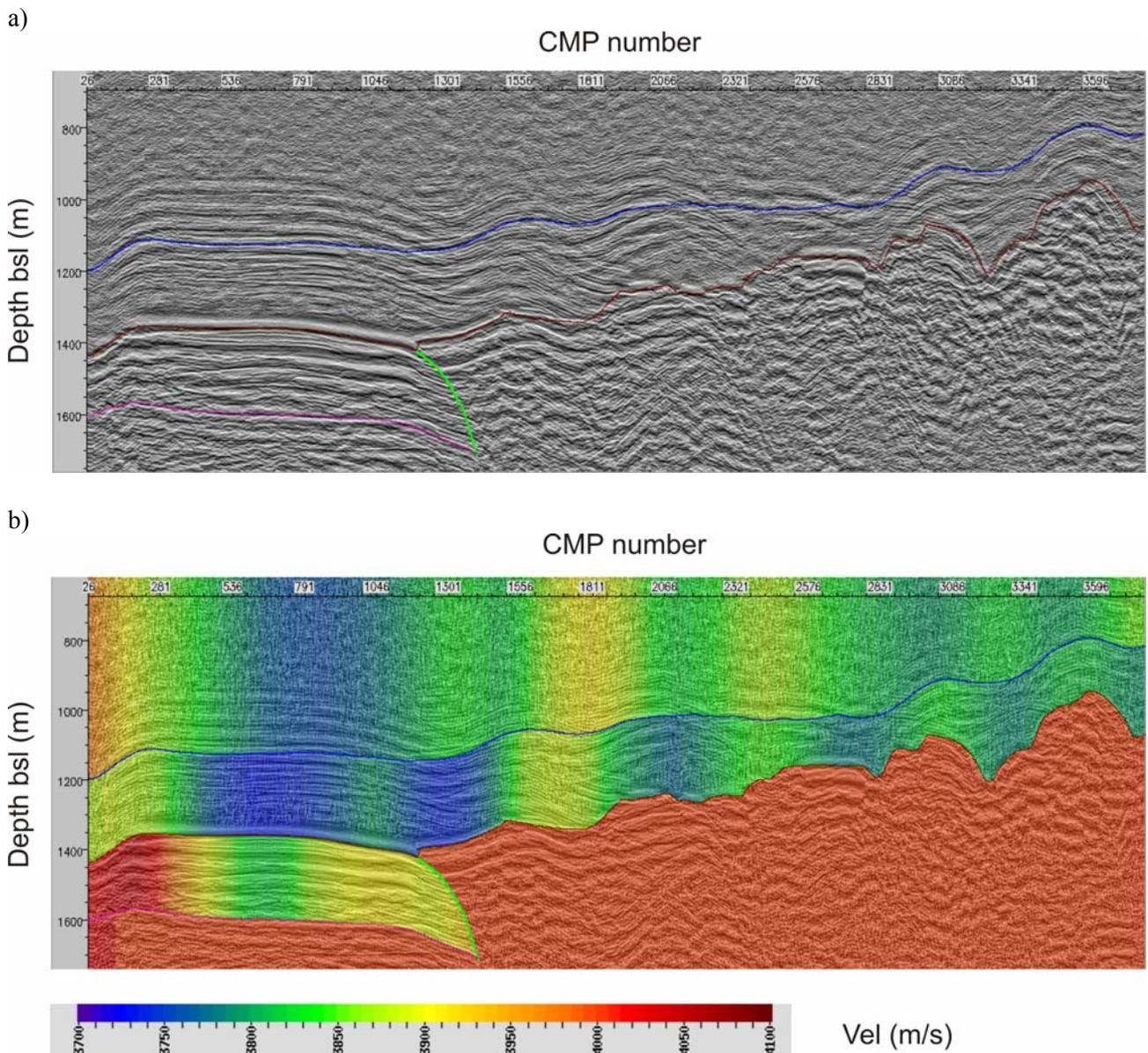
**Figure 3** – Final pre-stack Kirchhoff depth migration (a) and the final tomographic interval velocity model (b), where the vertical axis indicates the depth below sea level (bsl). The average glacier surface elevation is about 1300m and the CMP interval is 10m. Automatic Gain Control (AGC) is applied to enhance the weak englacial reflections.
