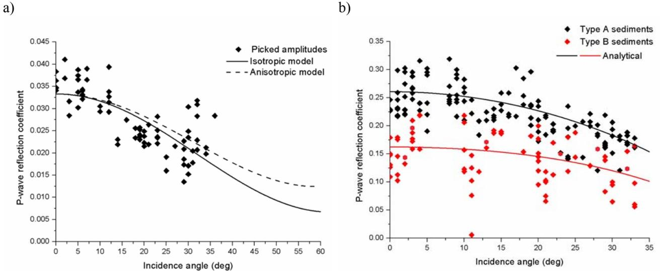
**Figure 5** – Best fit of the englacial reflection coefficients using the fracture model (a). Best fit of the bed P-wave reflection coefficients corresponding to type A sediments ( $V_P=2850$  m/s,  $V_S=1500$  m/s,  $\rho=2150$  kg/m<sup>3</sup>) and type B sediments ( $V_P=2400$  m/s,  $V_S=1100$  m/s,  $\rho=2100$  kg/m<sup>3</sup>) using the full Zoeppritz equations (b).
