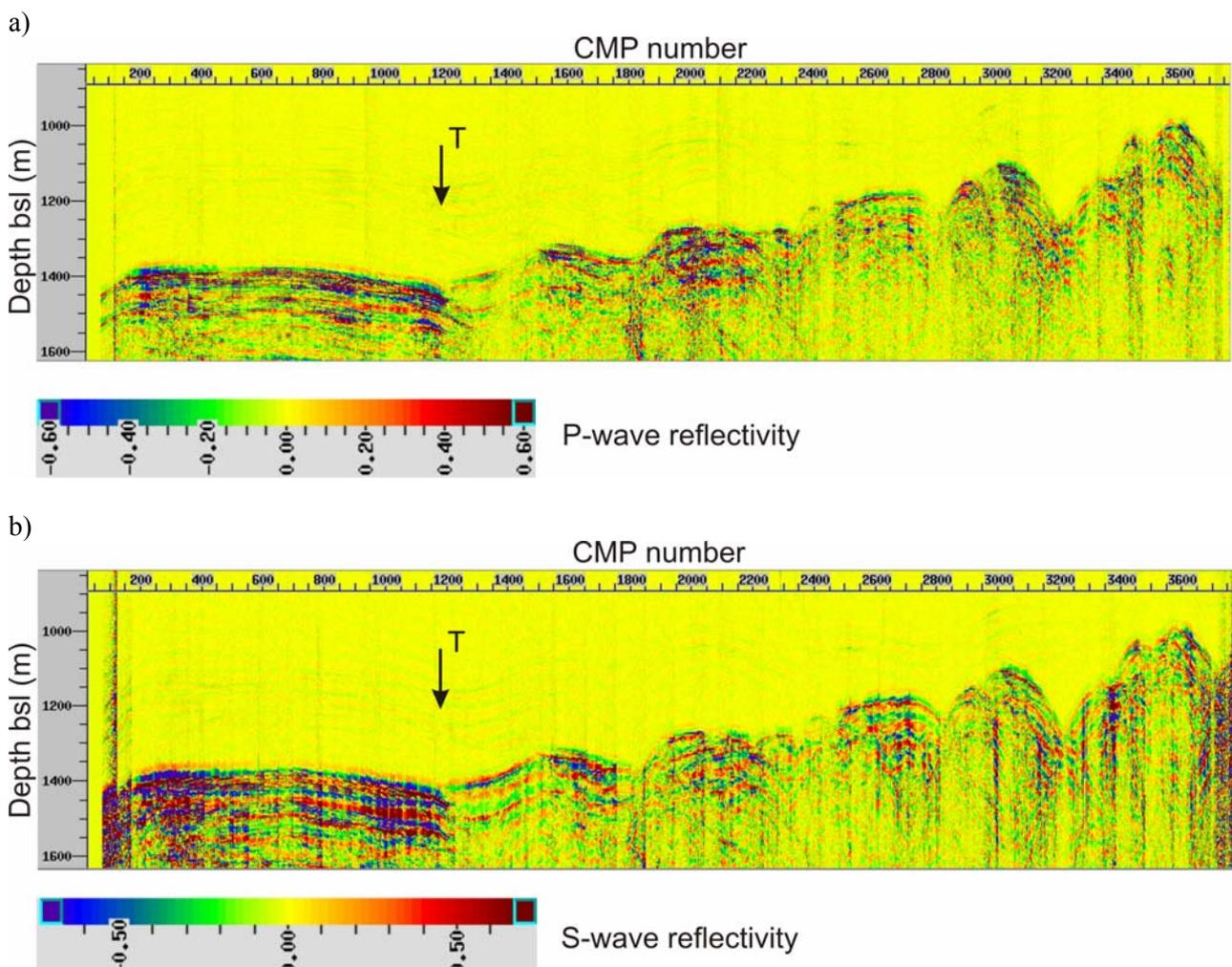
**Figure 4** – P-wave reflectivity (a) and S-wave reflectivity (b) sections, final results of the AVO inversion procedure, where the vertical axis indicates the depth below sea level (bsl). The average glacier surface elevation is about 1300m and the CMP interval is 10m. Indicated with T is a change in bed topography and a transition between two subglacial regimes.
